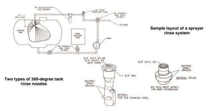
the valve is rinsed out, further reducing the chance for contamination of future pesticide mixes. To obtain the best results, practice using the rinse system by placing spray marker dye or food coloring in the spray tank. Using the rinse system, run three rinse cycles, making sure the water discharged from the nozzles is completely clear by the end of the third rinse.
